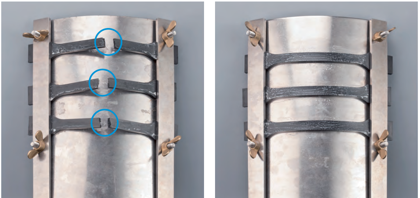
Fig. 5: Stress crack resistance test by means of the bent strip method, conducted analogously to DIN EN ISO 22088-3; Ultradur® B4300 G6 bk 5110 on the left and Ultradur® B4330 G6 HR bk 15045 on the right.
