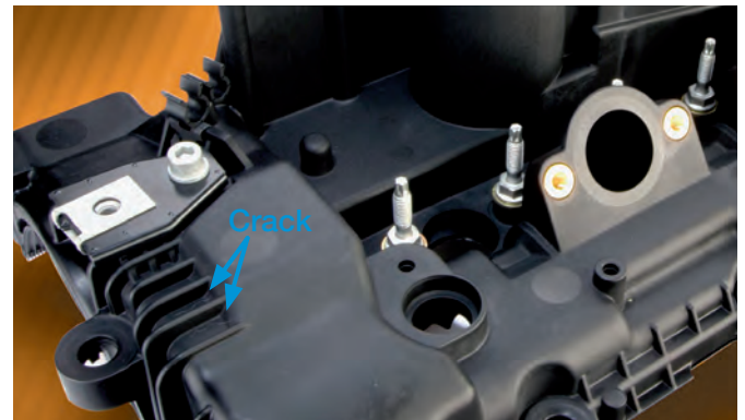
Fig. 4: Visible surface damage after short-term contact with sulfuric acid (2%).
