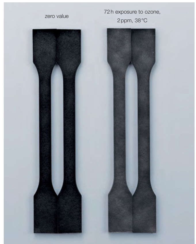
Fig. 55: Test specimens made of Ultramid® TKR 4355 G7 bk 564 before and after exposure to ozone. The color of the test bars faded slightly due to ozone exposure but the material properties remained largely unchanged
